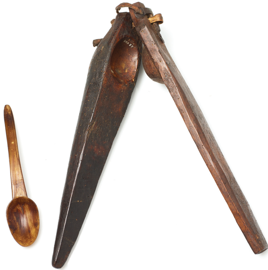
FIG. 5—Spoon mould of wood with leather hinge for shaping horn spoons (with Scottish horn spoon inset for scale). Used by travellers, Aberfeldy, Perthshire, Scotland. Nineteenth century. L. 45cm. Courtesy of Highland Folk Museum, Newtonmore, Scotland. Reg. No: SKA 59.
