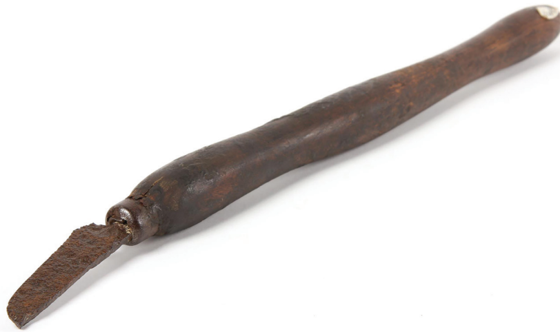
FIG. 3—Long handled knife for cleaning out the soft inside of the horn cores, its blade angled to fit into the curves, c.1790. L. 43cm W. 3.4cm. Photo: Museum of Design in Plastics, Arts University Bournemouth, courtesy of The Worshipful Company of Horners. Reg. No: WCHL:233.
