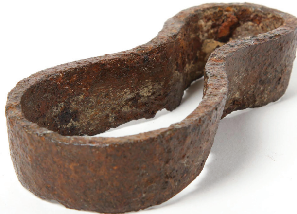
FIG. 4—Steel cutter for stamping blanks from prepared horn sheet, prior to reheating, moulding and finishing, while making horn spoons. The lowest edge is sharp, the top edge thick, for strength. L. 13cm, W. 2.5cm, D. 2.5cm. Photo: Museum of Design in Plastics, Arts University Bournemouth, courtesy of the Worshipful Company of Horners. Reg. No: WCHL:203.
