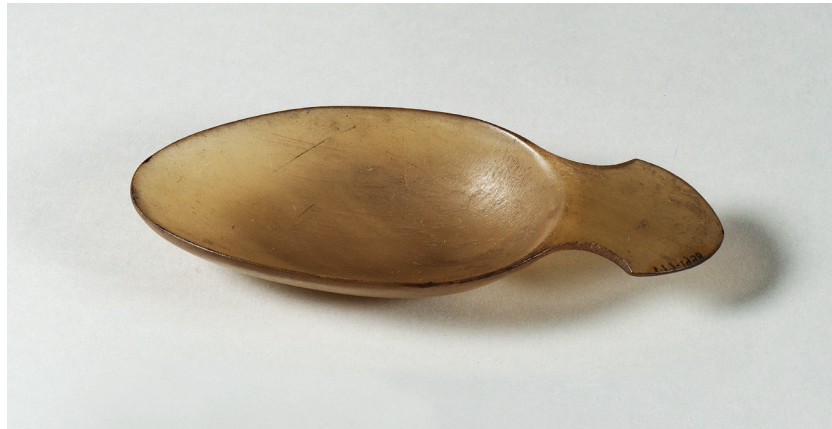
FIG. 13—Apothecary scoop made of horn sheet that was split into separate thin layers, prior to stamping out with a cutter (Fig. 4), then heated before moulding into the curved shape. Some double-ended examples had a pointed tip on the short end, useful to count pills or handle minute quantities, others were rounded like this. Nineteenth century. L.13.5cm, W.5.8cm. Courtesy Armagh County Museum. Reg. No: ARMCM.177.1958.
